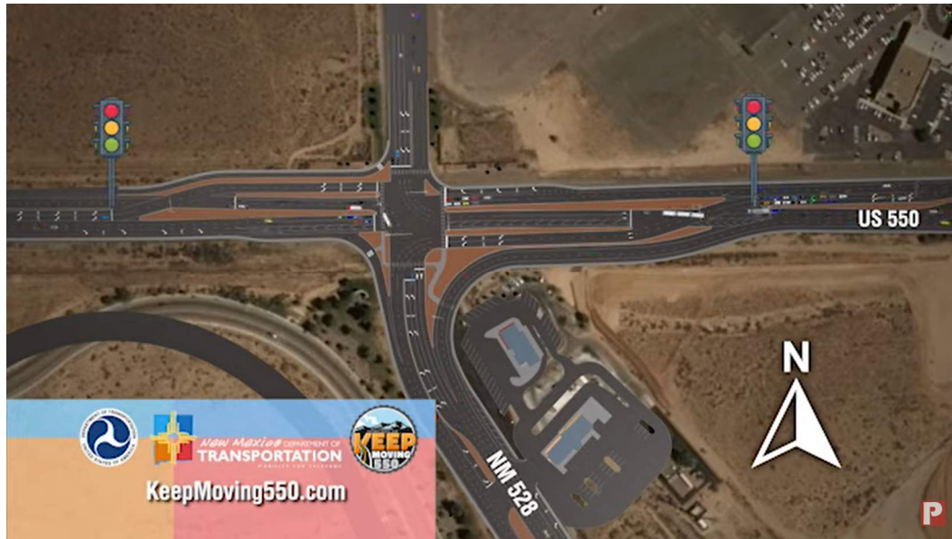
Figure 35: Continuous Flow Intersection Example
